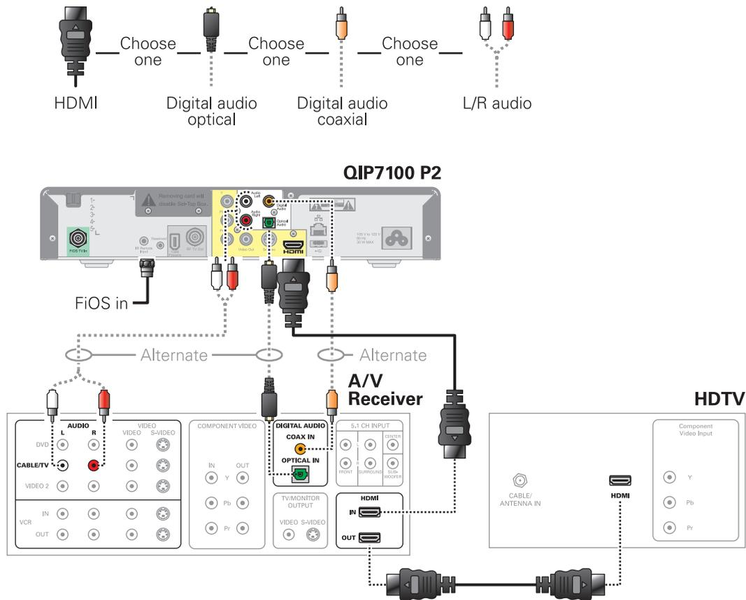
*Note: If the A/V receiver includes an HDMI input and output, the QIP7100's HDMI output can be connected directly to the A/V receiver's input and the A/V receiver's HDMI output directly to the TV. Because HDMI provides both video and audio output, no additional audio connections to the A/V Receiver and TV are required.*
