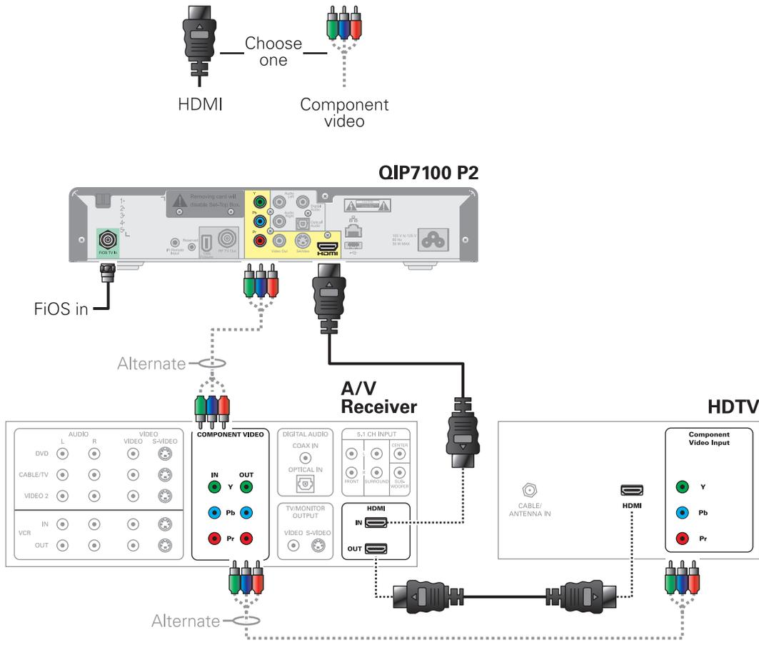
*Note: If the A/V receiver includes an HDMI input and output, the QIP7100's HDMI output can be connected directly to the A/V receiver's input and the A/V receiver's HDMI output directly to the TV. Because HDMI provides both video and audio output, no additional audio connections to the A/V Receiver and TV are required.*
