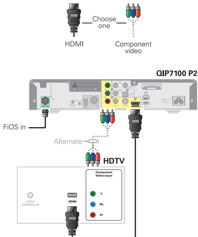
*Note: Because HDMI provides both video and audio output, no additional audio connections to the TV are required.*
