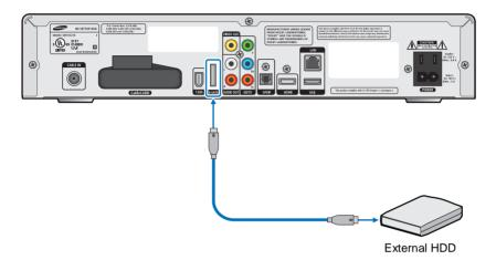
Connect the E-SATA port on rear of the STB with E-SATA port of external HDD by using E-SATA cable.
