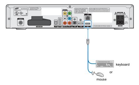
Connect the USB port on rear of the STB with USB devices by using USB cable.
