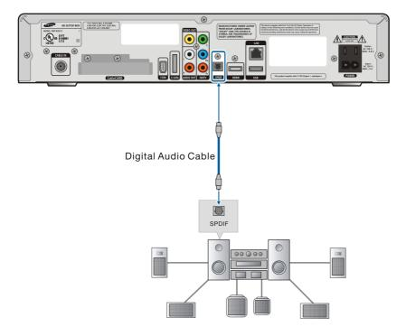
Using a Digital Audio cable (Optical cable), connect the **SPDIF** port on the rear panel of the STB to the **SPDIF** port on the digital audio (an amplifier or home theater that has a Dolby Digital decoding function).
